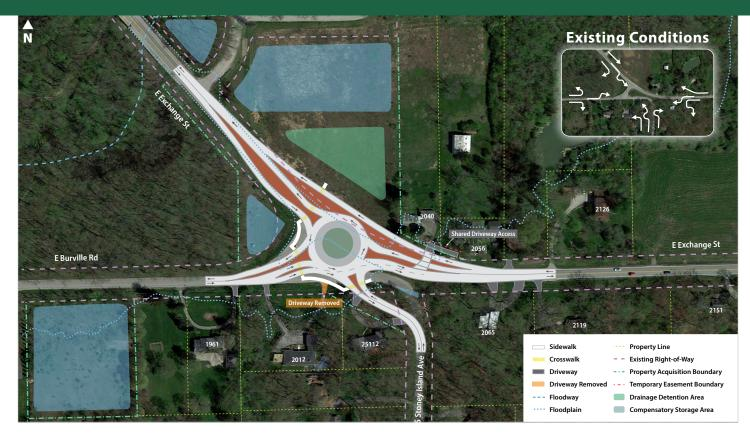
A roundabout is an unsignalized circular intersection and is considered one of the safest types of intersection design that operates with vehicles yielding upon entry. Roundabouts have been proven to be a safer design compared to intersections controlled by stop signs or traffic signals as they reduce fatal and serious injury crashes. This alternative is designed to have Stoney Island Avenue and Burville Road intersect Exchange Street at one intersection.
