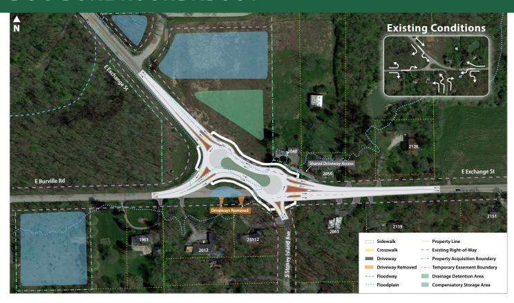
The Dog-Bone Roundabout functions the same as the Standard Roundabout with vehicles yielding on entry. To reduce impacts to the area, Stoney Island Avenue and Burville Road are kept separated. While it looks like two roundabouts combined, it functions as one intersection.
