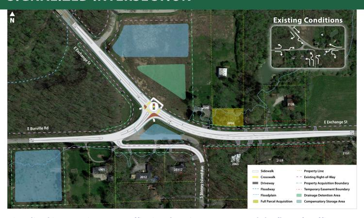
Signalized intersections use traffic signal equipment to control the flow of traffic improving operations compared to a stop controlled intersection.
